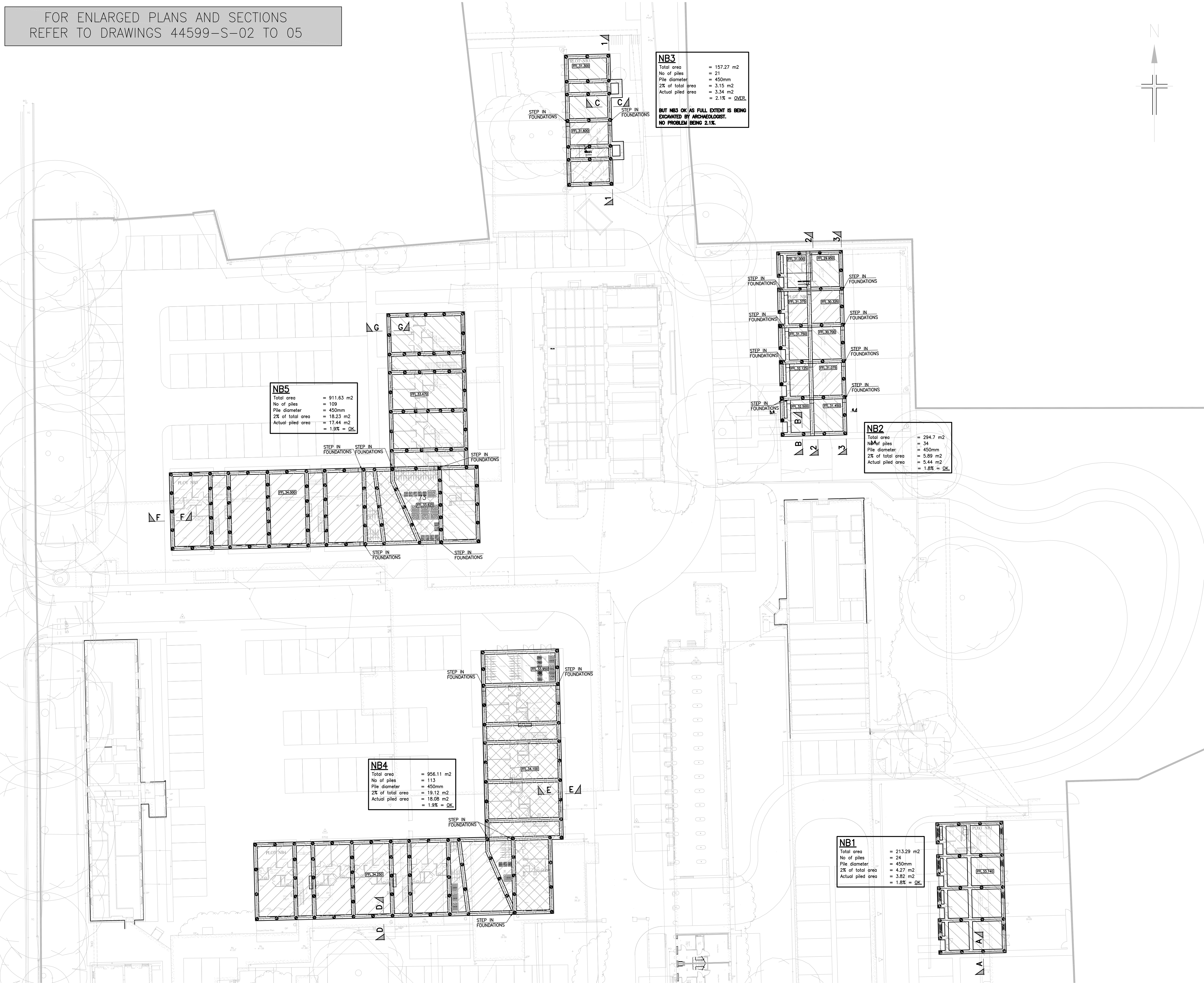
GROUND BEAM AND PILE GENERAL ARRANGEMENT FOR ALL AREA B1b PLOTS
