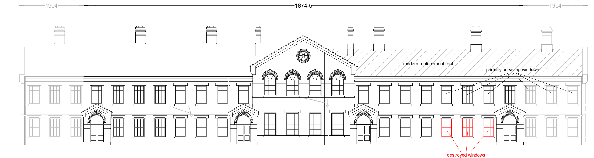
Fig 9 South-east elevation of the former Officers' Quarters, with alterations shown grey.
