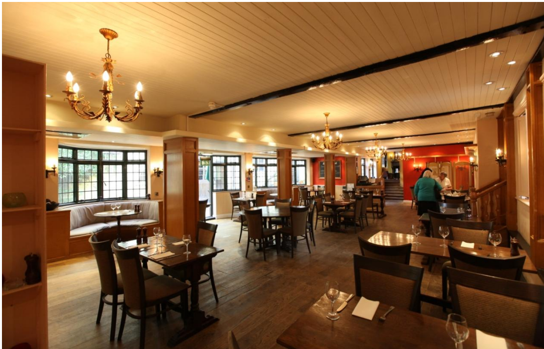
Illus. 19. The dining room in the western range (11), seen from the north with the bow-fronted extension of 1933-43 (12) on the left. This range dates from the mid-19 th century (1848-1876) with no evidence of the smaller, earlier structure which occupied its southern end. Each ceiling beam contains two mortises for vertical supporting posts, suggesting this space was designed as an open cart lodge divided into narrow bays.
