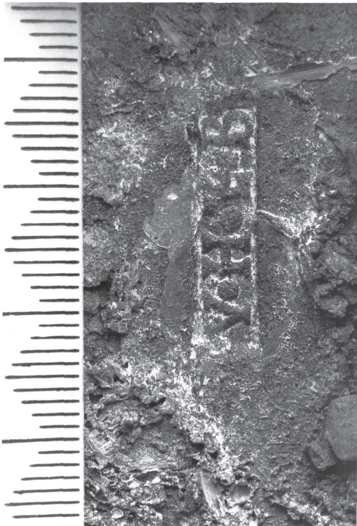
Plate 186: close-up of the stamp on the brass sheet with impressions of organic material on the surrounding corrosion (Ancient Monuments Laboratory; Crown copyright—reproduced with permission of the Controller of Her Majesty's Stationery office)
