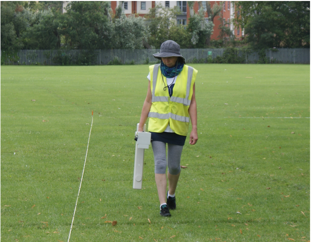
Figure 3. FM256 magnetometer in use. Marked guide string to operator's right.
