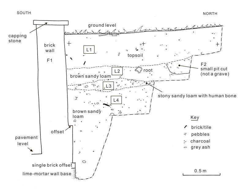
Fig 3: Test pit 1 section.
